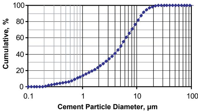
**Fig. 1:** Measured particle size distribution for the Type I/II portland cement used in the experiments (1 μm = 3.94 x 10<sup>-5</sup> in.)
