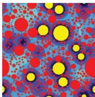
**Fig. 8:** Two-dimensional slice from three-dimensional simulated water availability distribution for IC mortar. Image size is 10 x 10 mm (0.39 x 0.39 in.); red indicates normalweight sand, yellow indicates LWA, and concentric rings of various shades of blue indicate hydrating cement paste within 0.1, 0.2, 0.3, 0.5, 1.0, and 2.0 mm (0.004, 0.008, 0.012, 0.02, 0.04, and 0.08 in.) of an LWA surface, respectively
