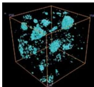
**Fig. 6:** Three-dimensional color-coded image of original data set subtracted from that obtained after 1 day of hydration. Aqua-colored volumes indicate regions where the LWA particles had lost water to the surrounding hydrating cement paste. The 3-D volume is 4.6 x 4.6 x 4.7 mm (0.181 x 0.181 x 0.185 in.)
