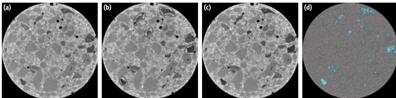
**Fig. 4:** Two-dimensional slices (13 x 13 mm [0.51 x 0.51 in.]) from 3-D microtomographic data sets corresponding to: (a) mortar immediately after mixing; (b) mortar after about 1 day of hydration; (c) mortar after about 2 days of hydration; and (d) color-coded original image subtracted from 1-day image. In the color-coded image, aqua indicates regions of drying and red indicates regions of wetting
