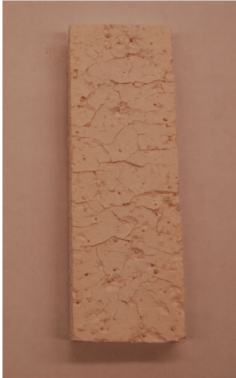
Figure 7. Cracking behavior of gypsum samples when heated at 700°C for Type R (Japan).
